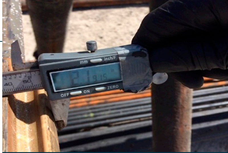
Guide OD measurement taken after operating 238 days resulting in a 10.53 to 13.53% guide wear.
