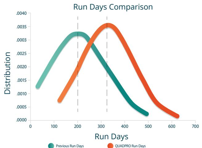
Figure 3: QUADPRO plungers are exceeding historical performance over a large sample size.
